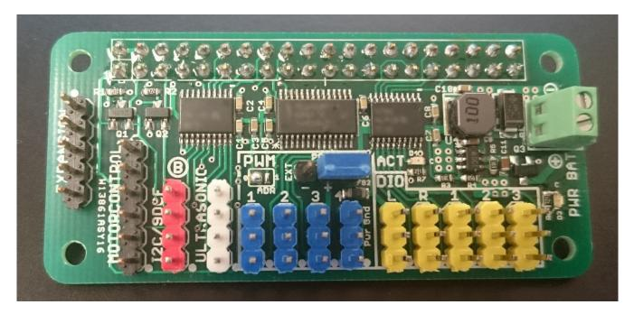
The PiBot Zero is a compact stacking daughter-card with the same footprint as the Raspberry Pi Zero. That can be used with the Raspberry Pi Zero, 2, or 3; it connects to the <u>Pi GPIO Header</u> to adapt the Raspberry Pi for robotics by providing:
