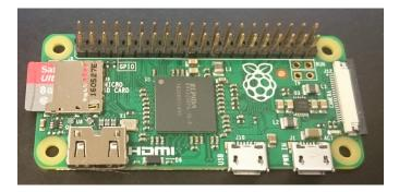
M2.5 x 11mm nylon standoffs may be used to securely mount the PiBot Zero to the Raspberry Pi Zero.
