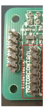
The PiBot Zero MOTORCONTROL interface uses two PWM channels and four GPIO channels to provide variable speed and direction control for each motor channel. If DC motor control functions aren't needed, the MOTORCONTROL connections can serve as additional digital inputs and outputs (DIO) and PWM control outputs which can be used to control servo motors.
